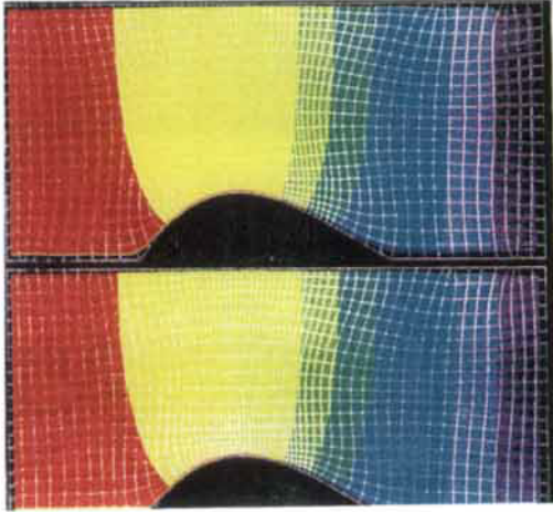
Plate 4. Cubic hill: contours of pressure
