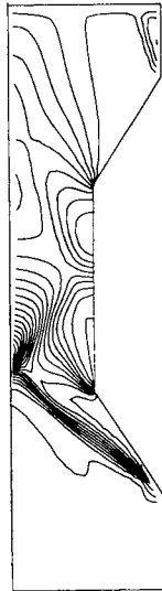
Figure 6. Wedge cascade: fine grid pressure field
