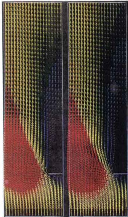
Plate 6. Vertical plate: velocity vectors and re-attachment streamline
