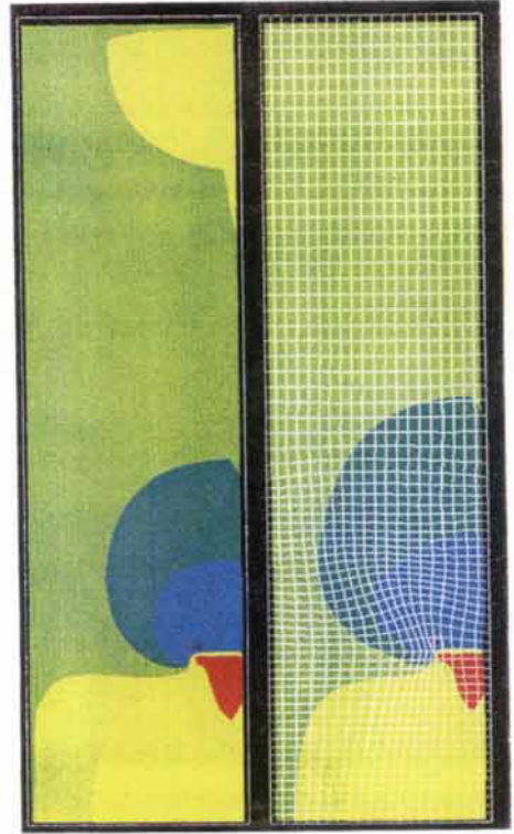
Plate 5. Vertical plate: grid before and after adaption including pressure fields
